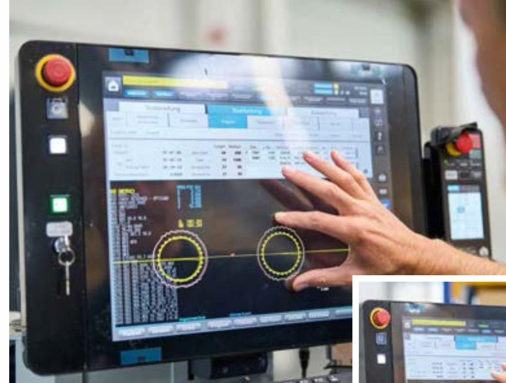
The highly user-friendly and intuitive multi-touch display of the MV1200S NewGen comes with freely configurable menus and can be operated using the gesture control familiar from tablet computers.
